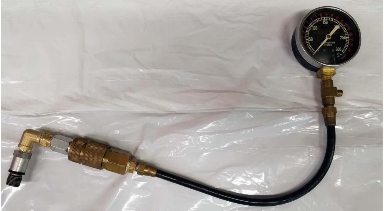
First off, thanks to Bill Griffin for the inspiration for adapting a standard compression tester to use on an 8N tractor with the hood still installed, and the use of air tool quick connects. This tutorial will show you how to adapt your compression tester so that it can be used in a tight ceiling area like the N tractor with the hood and gas tank left installed. You will be able to easily install the compression fitting into each spark plug hole in the tight ceiling area under the gas tank.
